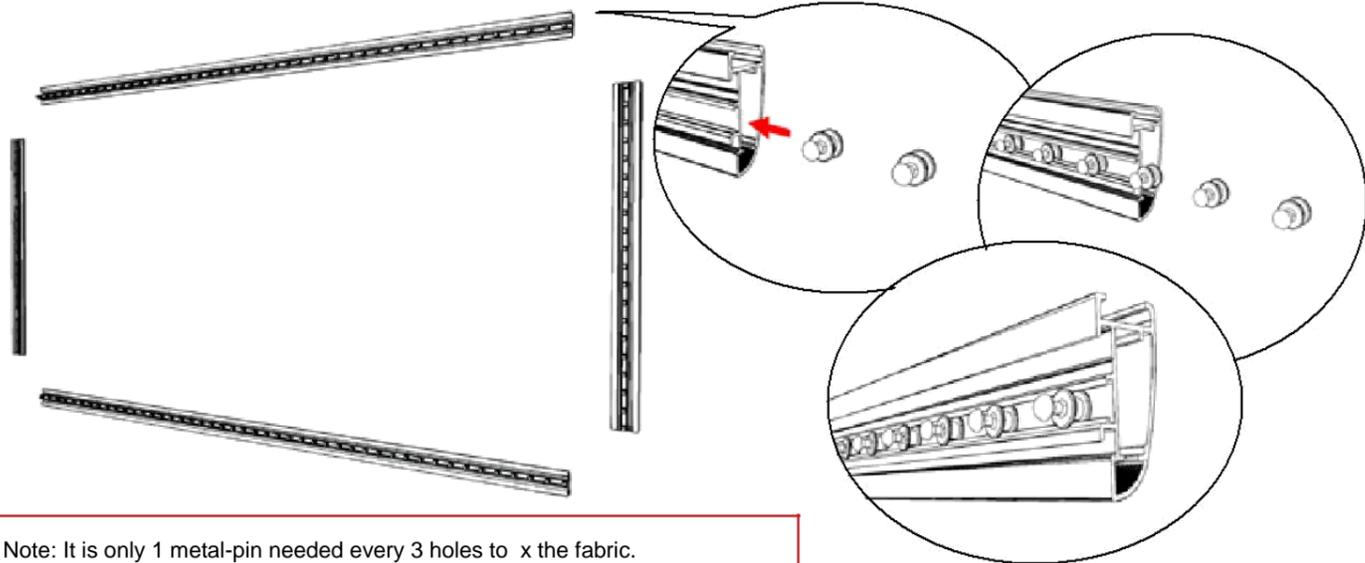
Note: It is only 1 metal-pin needed every 3 holes to x the fabric.
